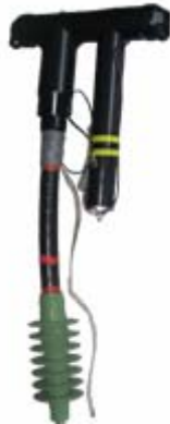
Fig.7: A 51 kV surge arrester during the routine test.
